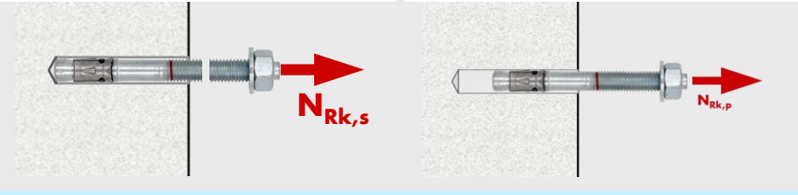
Verifications for the most loaded anchors
